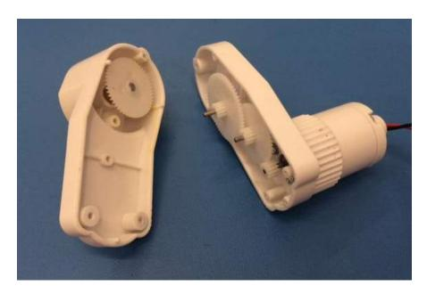
Use a No.1 Phillips Screwdriver to remove the 3 screws holding the gearbox together. Open the gearbox.
