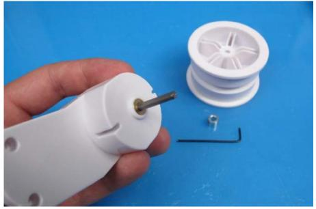
Use a 1.5mm Allen Key to loosen the set screw on the collar. Remove the collar and then remove the wheel from the gearbox. If the wheel does not separate easily, carefully pry the wheel away from the gearbox housing using a No. 2 Phillips screwdriver.
