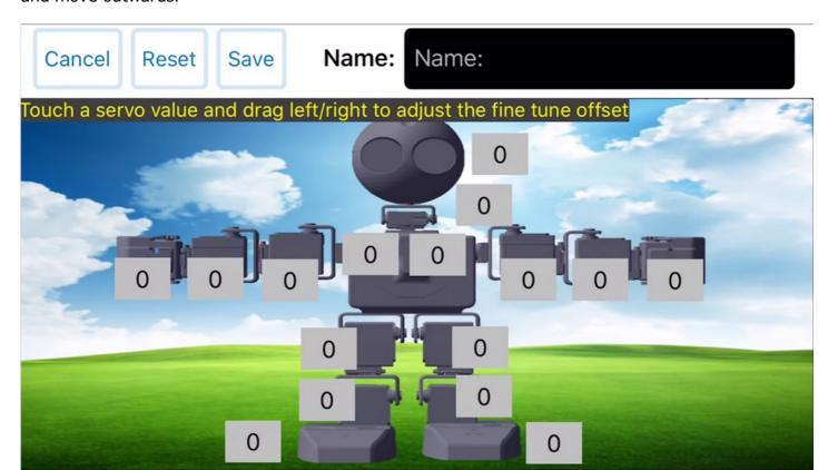
The robot grippers should not make a vibrating or grinding noise. Adjust the gripper servos as necessary to prevent damage.
